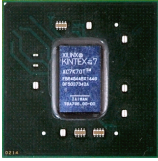
Figure 4: Image of a Kintex 7 XC7K70T device in a flip-chip BGA package [6]. The exposed silicon backside of the die can be seen in the middle of the package.
