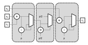
Fig. 5. Our optimized circuit for step (b) namely Yao garbling. The "+" gates refer to an integer addition circuit and "-" refers to an integer subtraction circuit. The trapeziods are multiplexers and the ">" refers to the circuit that outputs 1 if and only if the input is larger than p/2.
