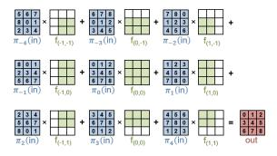
Fig. 9. Packed SISO Convolution. (Zeros in the punctured plaintext shown in white.)
