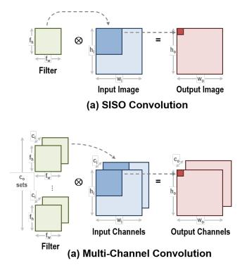
Fig. 2. SISO convolutions and multi-channel Conv layers
