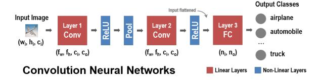
Fig. 1. A CNN with two Conv layers and one FC layer. ReLU is used as the activation function and a MaxPooling layer is added after the first Conv layer.
