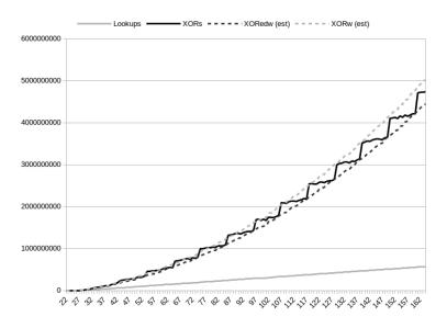
FIGURE 2. Comparison of the number of XORs in experiments with LowMC cipher to the estimated number of XORs by formulas (5) (upper bound) and (6) (lower bound).
