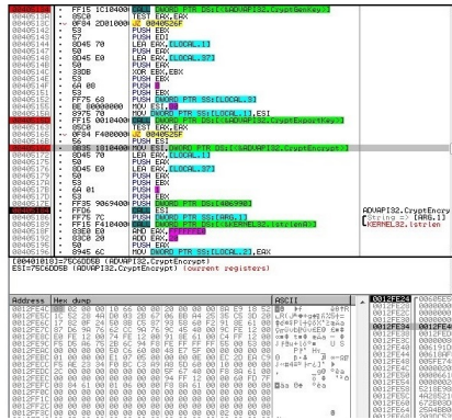
Fig. 12: Another AES key is generated, exported and encrypted using the embedded RSA key
