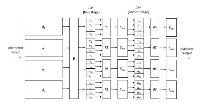
Figure 8: Description of the decrypt path of the IVP construction
