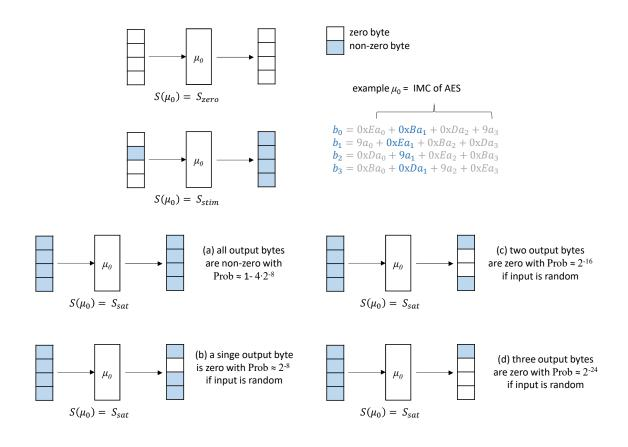
Figure 12: The states of a column mixing transformation
