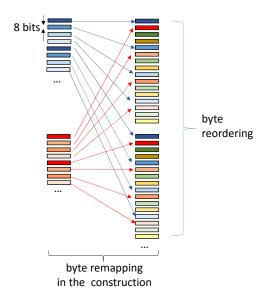
Figure 9: Byte remapping in the IVP construction
