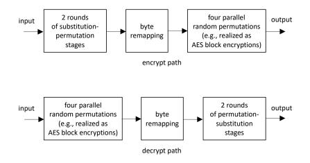
Figure 7: Overview of the encrypt and decrypt paths of the IVP construction
