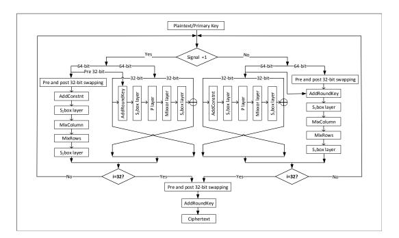
Fig. 1. Encryption procedure of SFN cipher [5].
