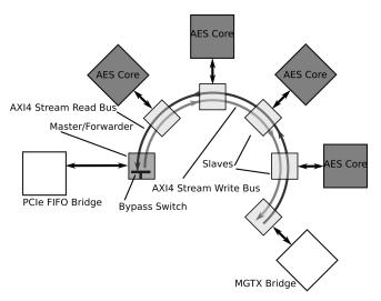
Figure 9. Network having AXI4 bus with PCIe FIFO bridge (master), 4 AES256 kernels (slaves) and 1 MGTX FIFO bridge(slave)
