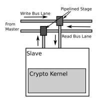
Figure 7. Pipe-lined Slave connector over AXI4 bus
