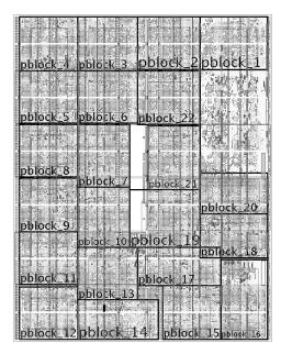
Figure 11. FPGA (xc6vlx240t) Floor plan for implemented 22 core AES256
