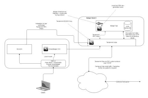
Fig. 1. Our System Architecture (only single threshold node shown)
