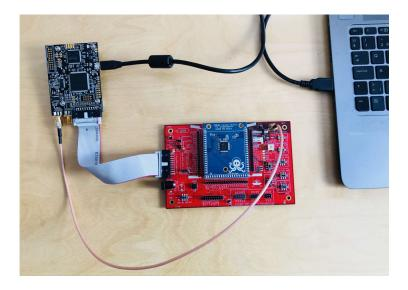
Fig. 2. The second board with ATxmega128D4 microcontroller (right) connected to the ChipWisperer (left).
