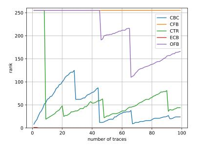
**Fig. 5.** Results of the 1st key byte ranking for *n* traces of XMEGA1 AES in different modes of operation by MLP trained on XMEGA1 AES-ECB, for  $1 \le n \le 100$ .
