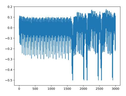
Fig. 6. The first 3000 data points of a power trace of XMEGA1 during the execution of AES-ECB.
