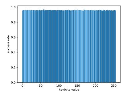
**Fig. 3.** Probability of recovering the 1st key byte from a single trace of XMEGA1 AES by MLP trained on XMEGA1 AES for different byte values.
