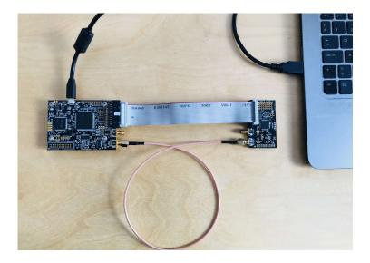
Fig. 1. The first board with ATxmega128D4 microcontroller (right) connected to the ChipWisperer (left).
