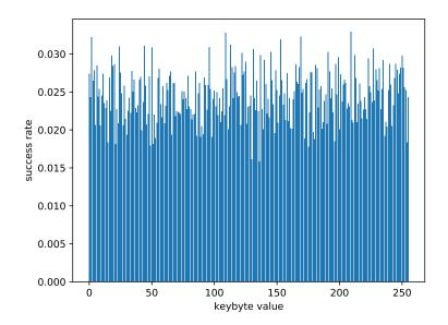
**Fig. 4.** Probability of recovering the 1st key byte from a single trace of XMEGA2 AES by MLP trained on XMEGA1 AES for different byte values. Note that the range of Y-axis is [0;0.03], while in Fig. 3 it is [0;1].
