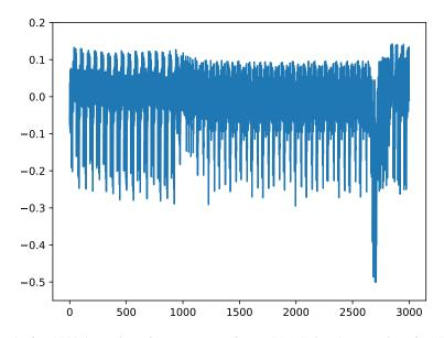
Fig. 8. The first 3000 data points of a power trace of XMEGA1 during the execution of AES-CTR.
