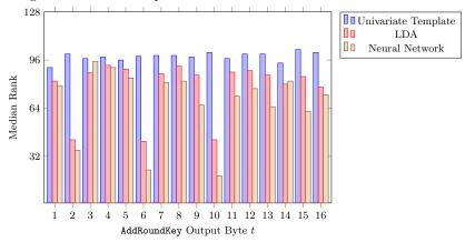
(b) Plot showing the classification results of the  ${\tt AddRoundKey}$  output using Median Rank as a performance metric
