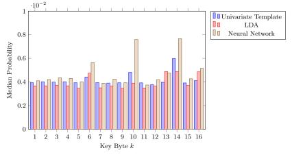
(c) Plot showing the classification results of the key bytes using Median Probability as a performance gnetric
