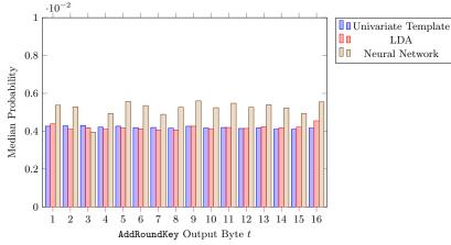
(b) Plot showing the classification results of the  ${\tt AddRoundKey}$  output using Median Probability as a performance metric
