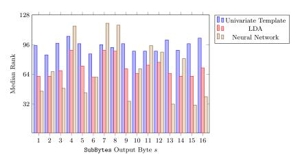
(a) Plot showing the classification results of the  ${\tt SubBytes}$  output using Median Rank as a performance metric
