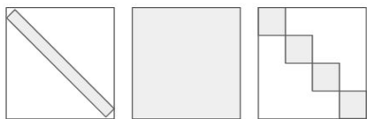
Fig. 2. In left we represent the number of coefficients to compute in case of gradient descent, in middle the full Hessian matrix and in right our block-wise approach. Note that just the elements in grey are computed.
