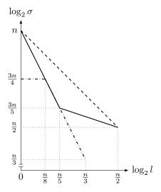
Fig. 2: The threshold number of the total length of the encryption queries  $\sigma$  as a function of l, where the number of faulty queries  $\mu$  is fixed as a small constant. The solid line is the bound for SCM, while the dashed (resp. dash-dotted) line is the bound for AES-GCM-SIV in the ideal cipher (resp. multi-user PRP) model.
