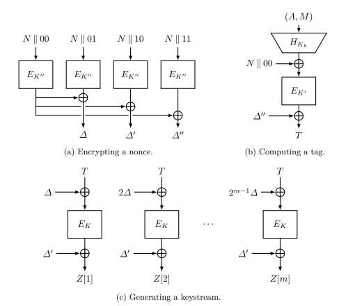
Fig. 3: The SCM mode based on H and E using a key  $(K_h, K, K', K'')$ .
