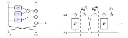
Fig. 5. SIMON/Simeck round function [13]. Fig. 6. SIMON/ Simeck one round extension for pre-whitening key.
