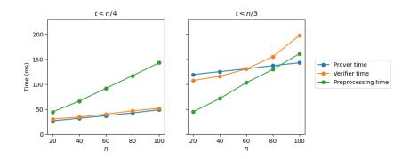
**Fig. 7.** Timing on the 10-block SHA256 circuit with  $t = \lfloor (n-1)/4 \rfloor$  and  $t = \lfloor (n-1)/3 \rfloor$  respectively. The base field is  $\mathbb{F}_{2^7}$  and for t < n/3 the extension field is  $\mathbb{F}_{2^{91}}$ .
