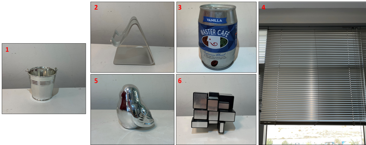
Fig. 6. The lightweight reflective objects used to recover sound: (1) decorative bucket, (2) smartphone stand, (3) iced coffee can, (4) Venetian blinds, (5) bird statuette, (6) Rubik's Cube.
