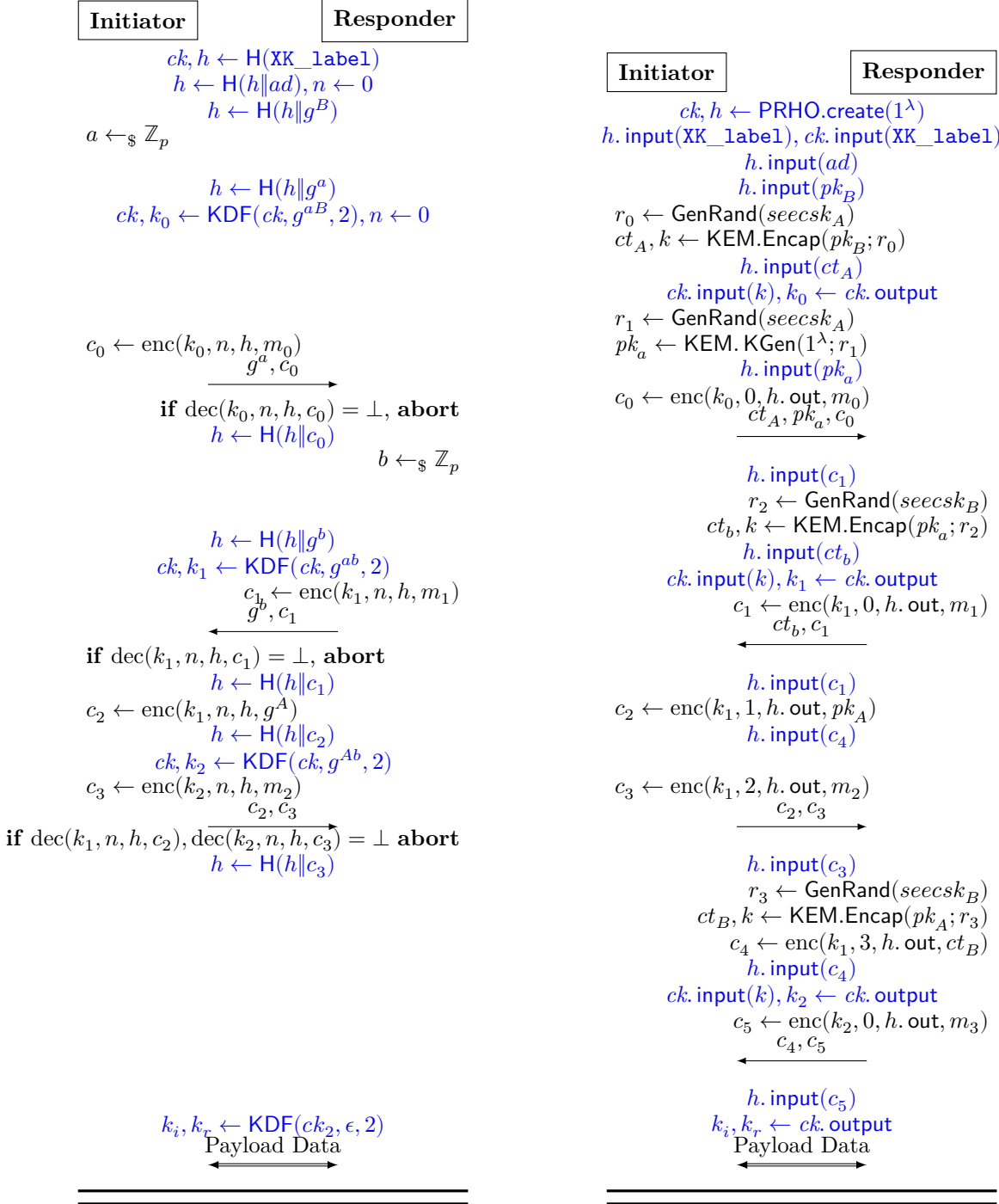
Figure 12: The XK patterns of classical Noise (left) and PQNoise (right). For reasons of space we use the following conventions here: highlighted actions are performed by both parties as soon as they receive all necessary values to perform the computations in question. If any decryption- or decapsulation-algorithm returns \perp , the party in question aborts the protocol.
