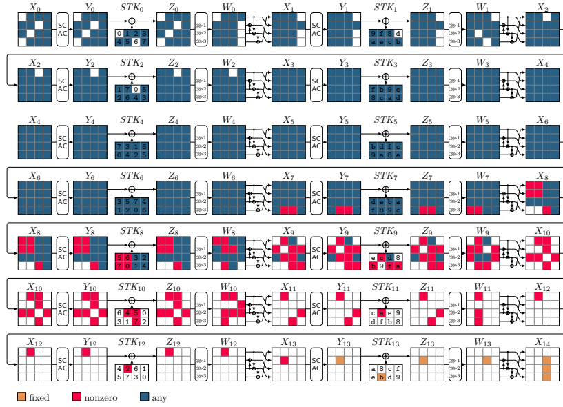
Fig. 26: ZC-Integral distinguisher for 14 rounds of SKINNY- n-3n . STK[0] is active at most three times. X_{14}[6] \oplus X_{14}[10] \oplus X_{14}[14] is balanced. Data complexity: 2^{7 \cdot c} .
