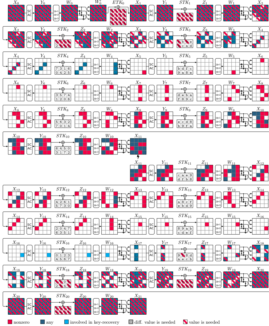
Fig. 9: ID attack on 21 rounds of SKINNY- n-3n . |k_B \cup k_F| = 42 \cdot c , c_B = 15 \cdot c , c_F = 15 \cdot c , \Delta_B = 16 \cdot c , \Delta_F = 16 \cdot c .
