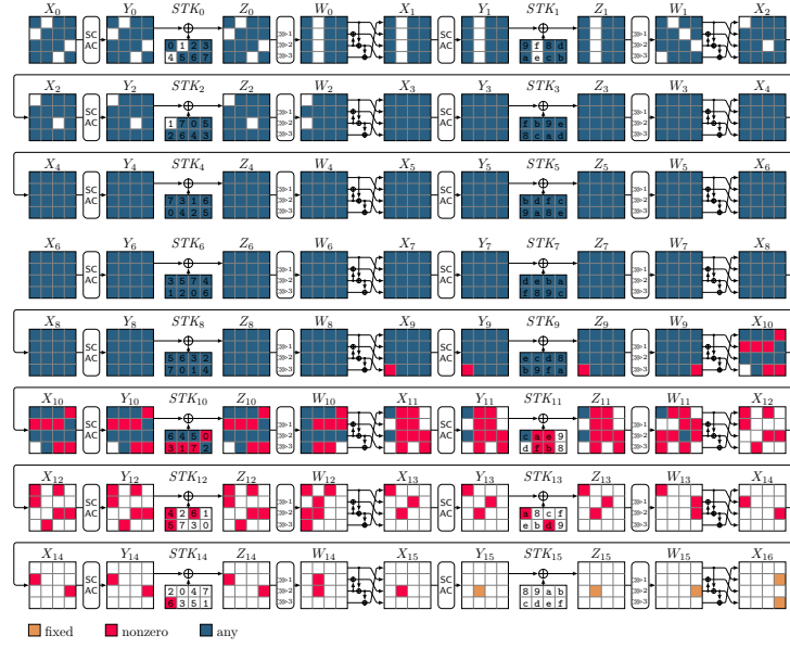
Fig. 29: ZC-Integral distinguisher for 16 rounds of SKINNYe/SKINNYe-v2. STK[1] is active at most four times. X_{16}[7] \oplus X_{16}[15] is balanced. Data complexity: 2^{32} .
