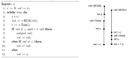
**Figure 1** A randomized consensus algorithm on the left, and an execution template  $(c_0 \in \{0, 1\})$  on the right, which represents the executions of an adaptive adversary which disallows termination.
