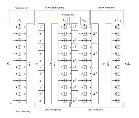
Figure 2: One round of the XHash8 permutation
