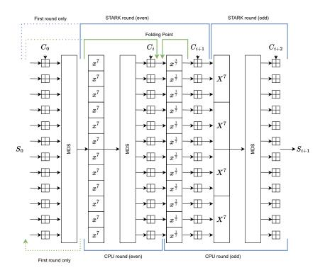
Figure 1: One round of the XHash12 permutation
