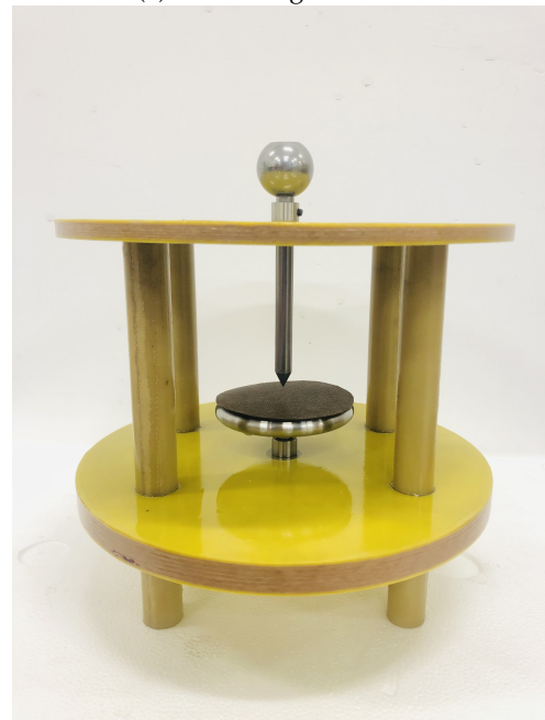
(b) Physical map of simulated fuel tank and electrode support
