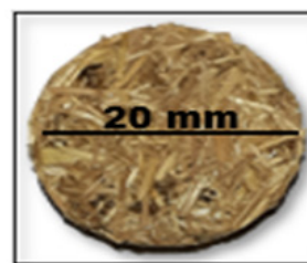
Figure 1: Photograph of fabricated composite with rice straw and latex.
