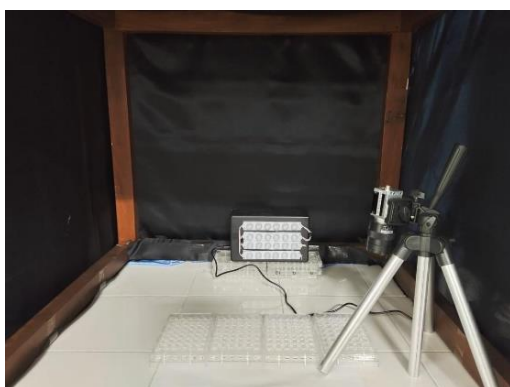
Figure 2. Illustration of a black box cover so that other lights do not interfere with the camera on the top and the light on the bottom design by author.
