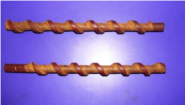
Fig. 4. Photograph of helical screw tape inserts
