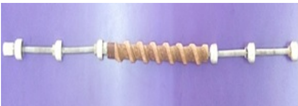
Fig. 5. Picture of compound insert case 1 (C1)
