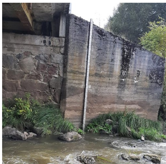
Fig. 2. HP Ulyanovo on the river Instruch: the position of the measuring rail on the bridge support. Photo of the authors during the summer-autumn low water period (08.10.2022).
