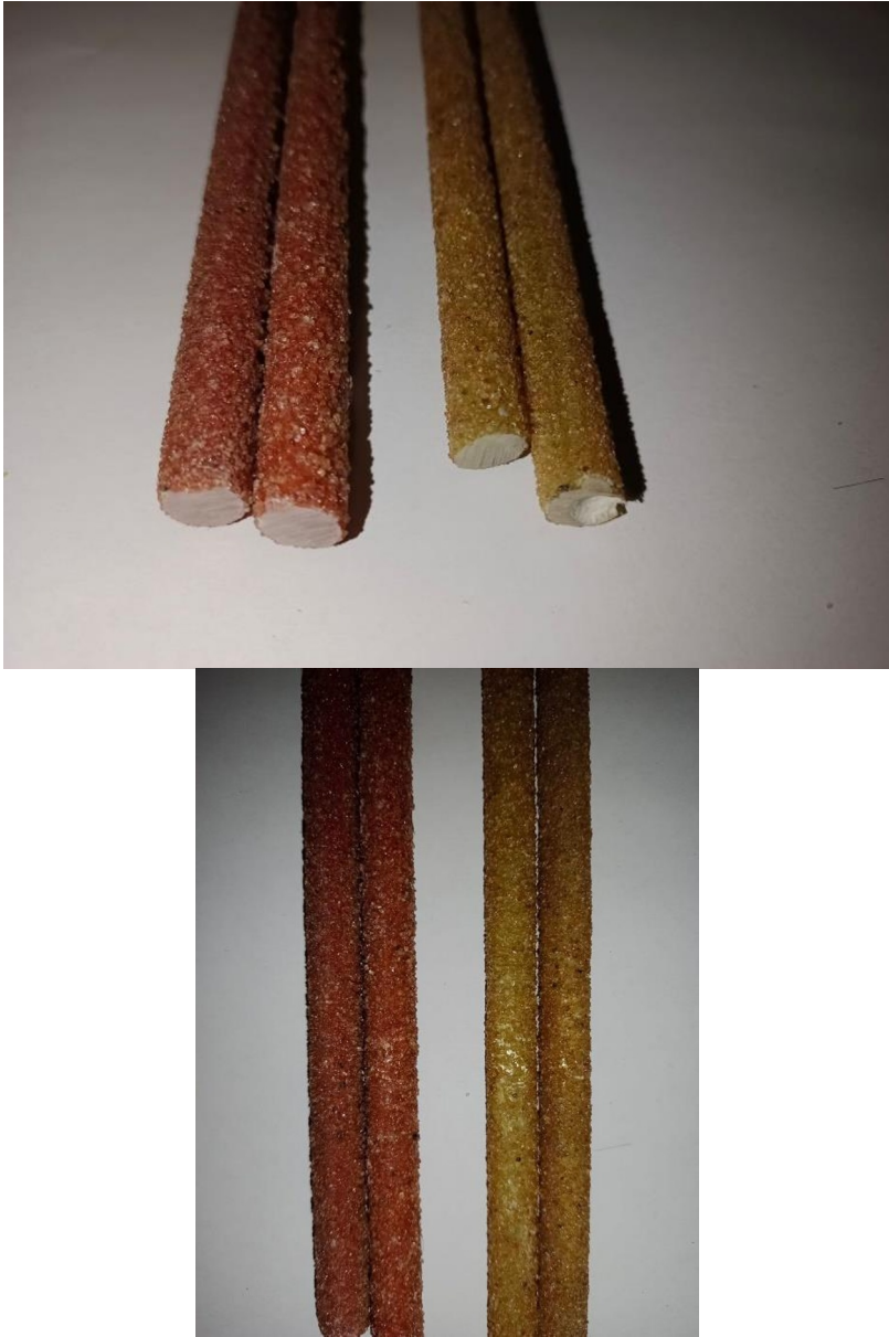
Fig. 8. Samples of glass-composite reinforcing bars obtained on the basis of colored and uncolored epoxy binder
