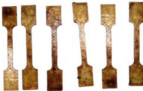
Fig. 7. Samples made of cured binder EDI-75 after exposure for 28 days in 40% NaOH aqueous solution at 90°C.
