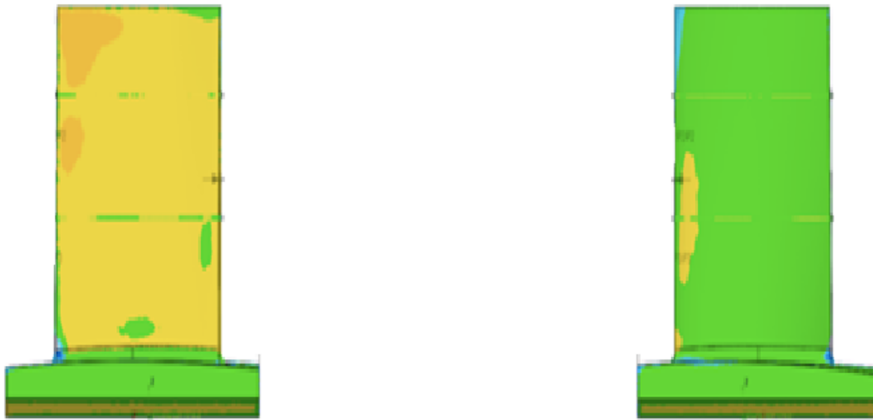
Fig. 15a. Inspection of blade geometry and deflection in the longitudinal section.
