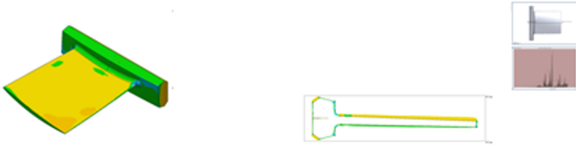
Fig. 15a. Inspection of blade geometry and deflection in the longitudinal section.
