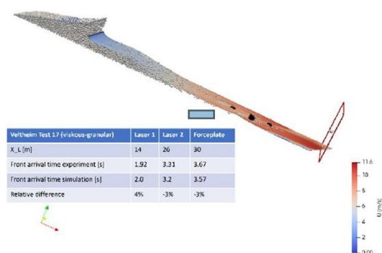
Fig. 8. Side view perspective of the resolved CFD-DEM simulation of debrisInterMixing coupled with Yade, DIMYade, and a table comparing simulation and experiment.
