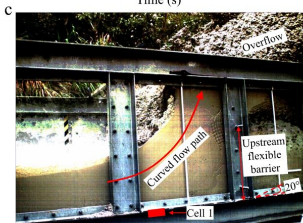
Fig. 4. Measured flow basal stresses and flow depth in [7] for (a) test V6-B1; (b) test V6-B2. (c) Run-up impact mechanism on the upstream flexible barrier for test V6-B2.
