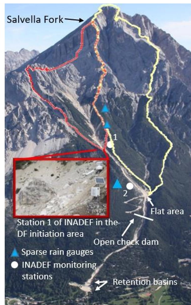
Fig. 4. The site of Rovina di Cancia with the rain gauges (triangles, dark of ARPAV and white of INADEF) and the numbered monitoring stations (circles) used for testing the WGA. The red and yellow lines identified the basins drained by the initiation area and the mouth of Bus de Diau Creek, respectively.
