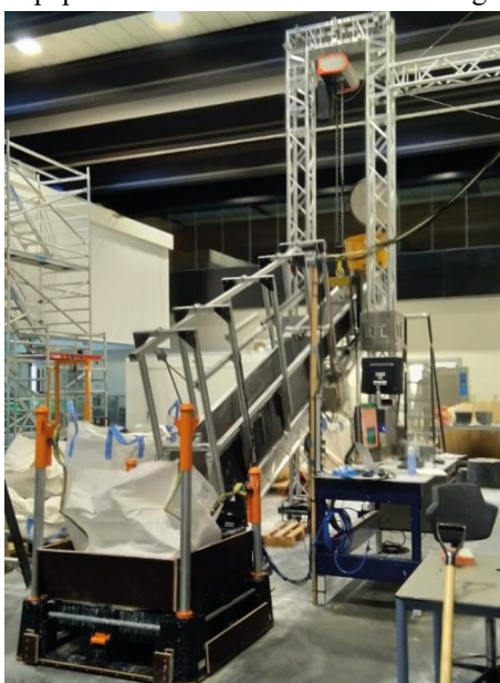
Fig 1 Flume set-up. The yellow cylinder in the top right is the sediment-mixing tank. In the lower half of the flume, beneath the metal frame, the erodible bed is present.
