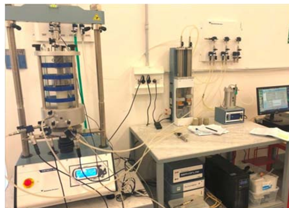
Fig. 3. Triaxial testing machine for unsaturated soil.
