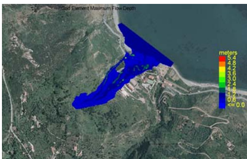
Fig. 8. Maximum flow depths for c_v = 0.569 and T_r = 50 years.
