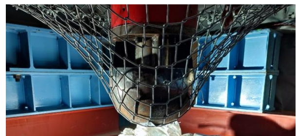
Fig.3. Large displacement of normal chain link.
