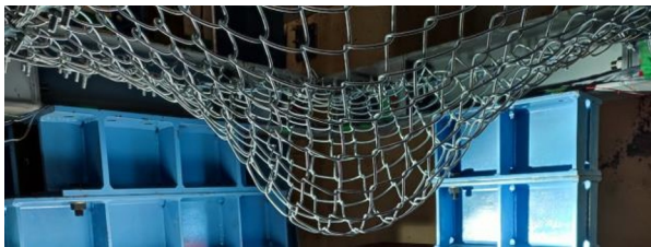
Fig. 4. Displacement of high-performance chain link after weight removal.
