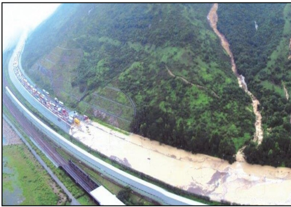
Fig. 1. Landslide debris caused the closure of North Lantau Highway, the critical transport corridor to the Hong Kong International Airport, in June 2008.
