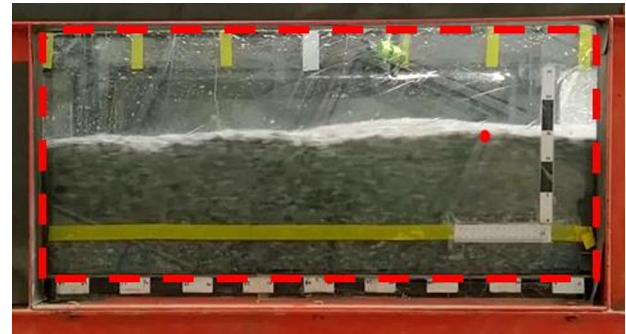
Fig. 4. Side profile of the experiment. The dashed outline indicates ROI for image analysis and the dot indicates the particle being tracked.
