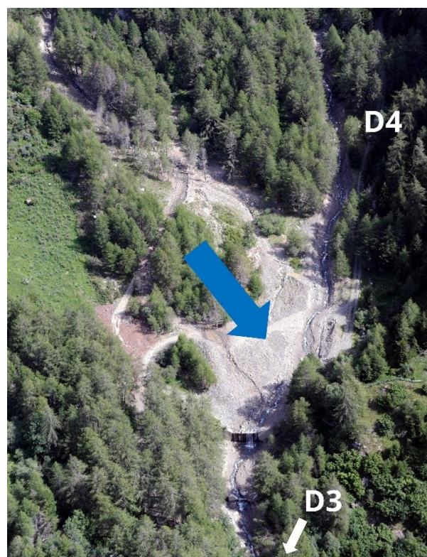
Fig. 2. Aerial photo of the channel between D4 and D3; the blue arrow indicates a low-slope, partly unconfined sector of the channel.
