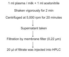
Fig. 1. Flow chart for extraction of ceftizoxime from plasma and milk.
