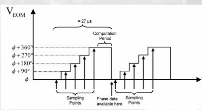
The phase shifting is carried out by applying a stepped waveform to the EOM (see left). After the 5 shifts have carried out, the phase data is calculated by the DSP using the Schwider-Hariharan phase shifting algorithm.
