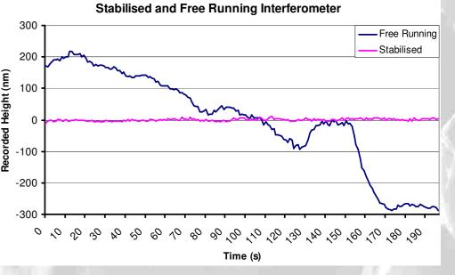
The repeatability of the instrument was investigated by measuring the response of the stabilised interferometer 1000 times.
