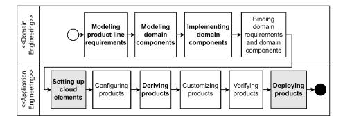
Fig. 5. New SPL implementation process (UML activity diagram).
