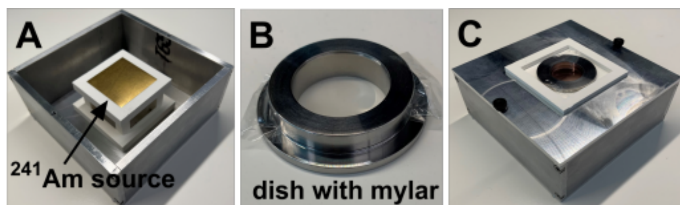
Figure 1. Components of the \alpha -particle irradiator before the addition of a shutter. Photo A depicts the \alpha source, B shows the cell dish with mylar to adhere to, and C is the complete assembly.
