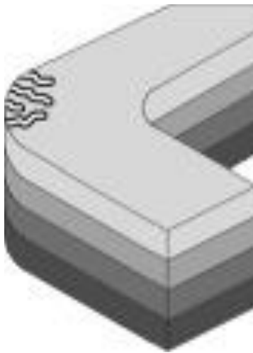
Figure 2.19 Tearing and texture issues with tight curvatures in 3DCP (Roussel, 2018)
