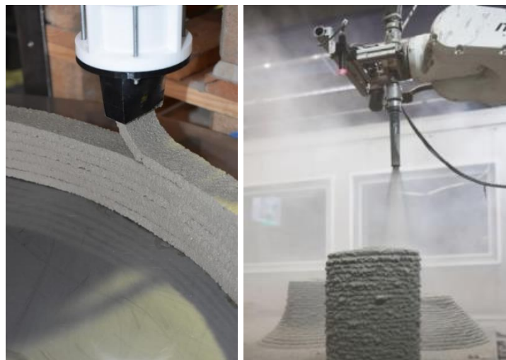
Figure 2.3 3D Concrete Printing through extrusion of concrete (left), Spray-based “Shotcrete” 3D Concrete Printing through spraying of concrete (right)
