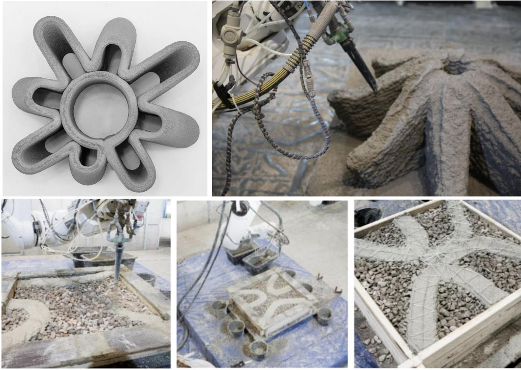
Figure 3.20 Examples of layer sizes and layer curvatures (Anton et al., 2020; Lachmayer et al., 2021; Mai et al., 2021)
