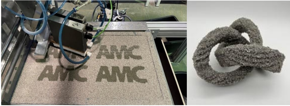
Figure 2.9 Selective paste intrusion where an aggregate layer has cement paste applied in areas to be hardened
