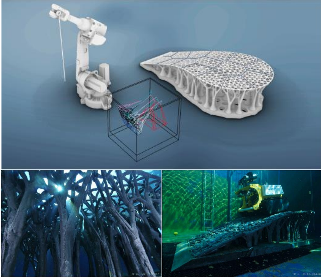
Figure 2.6 Visualization of artificial reef module and printing setup: Module is printed in carrier bed and banded together into a slab.
