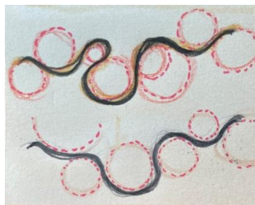
Figure 3.21 High versus low curvature as an approximation for minimum feature size
