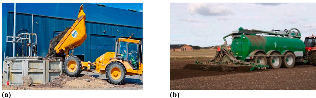
Fig. 4. (a) Pre-treatment at Solrød Biogas Plant, separating seaweed and sand, and (b) N rich digestate distributed as fertilizer on nearby farms (Coastal Biogas, 2020b).
