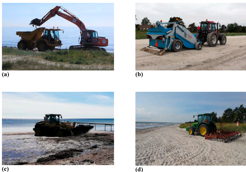
Fig. 2. (a) An excavator with a large front shovel and a dump truck; (b) a beach cleaning machine; (c) a loader tractor; and (d) a tractor with a large metal rake connected to it (Coastal Biogas, 2020b).
