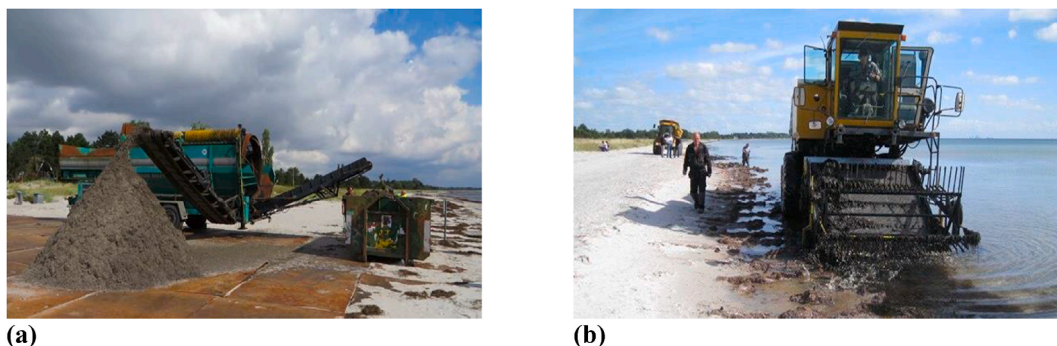
Fig. 3. (a) Container and drum sieve separating sand from seaweed; (b) the Halmstad prototype harvester trialled by Solrød Municipality (Coastal Biogas, 2020b).
