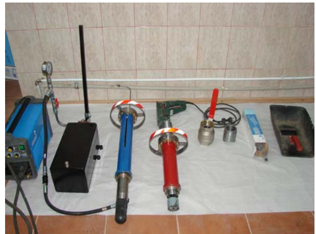
Figure 5 The equipment for interventions at pipes under pressure Dn 80
