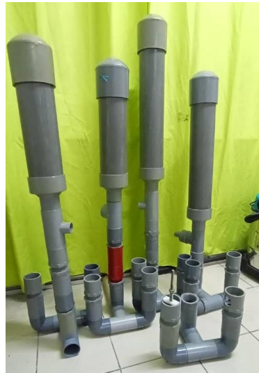
Fig. 7 - Ramp pump used in this project
