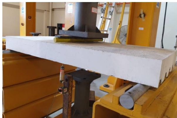
Fig. 4 - Three-point bending test of slab specimens
