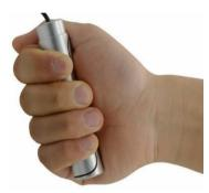
Fig. 4 - Handgrip force transducer
