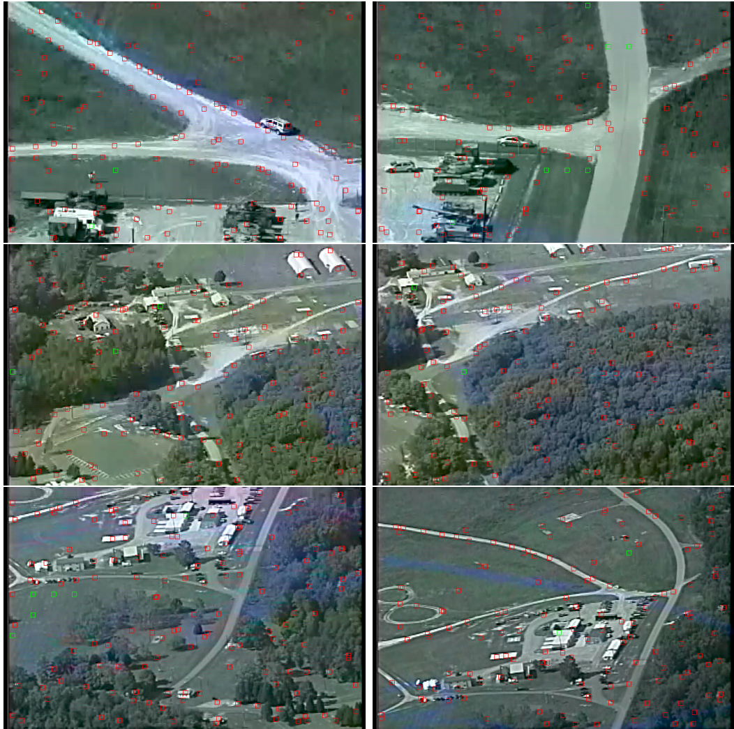
Figure 5.4: Boxes drawn around ST points for different frames of the sequence. Green squares represent homogeneous points
