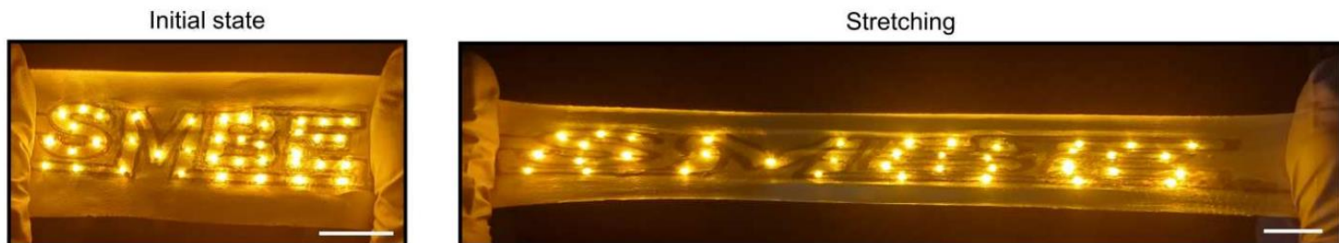
Figure 3.6: Photographs of light-emitting diode arrays, interconnected with conductive traces of porous EGaIn composites
