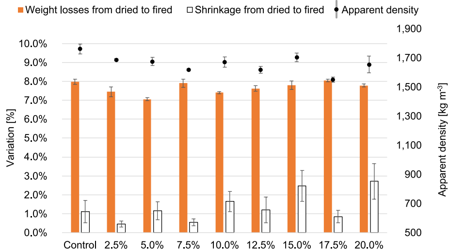
Fig. 7. Apparent Density of fired samples, firing losses and firing shrinkage.
