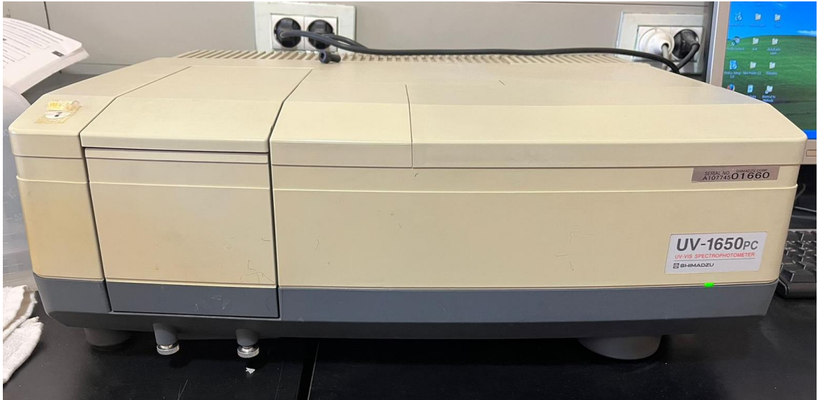
Figure 3-5: Shimadzu Ultraviolet-Visible (UV - Vis) Spectrophotometer (Model UV-1650)
