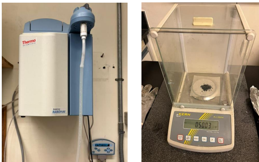
Figure 3-6: Nano pure UV Water Treatment Unit and Kern Analytical Balance
