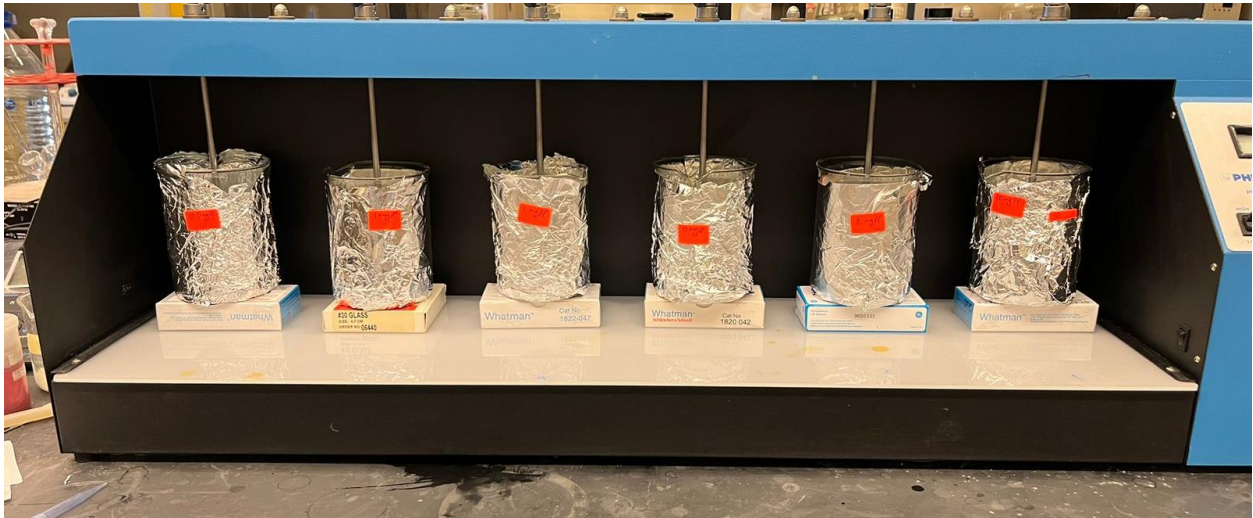
Figure 3-7: Jar Test Apparatus Used for Mixing Different Concentrations.
